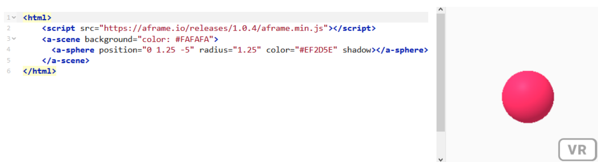
Figure 4. The output source code and the result of the simple programme running in A-Frame.
