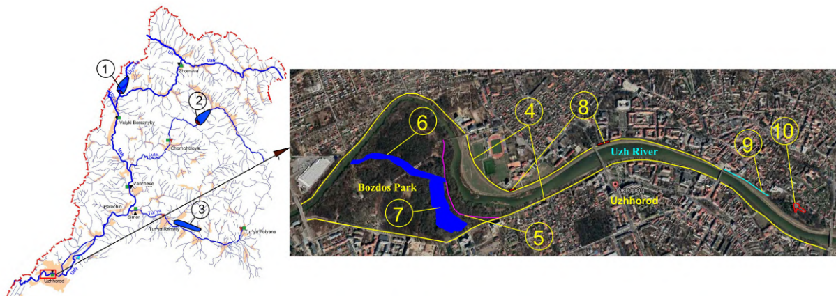
Figure 6. Flood mitigation measures: 1, 2 – dry retention reservoirs; 3 – polder; 4 – dyke 1% probability; 5 – dyke 10% probability; 6 – old river bed; 7 – oxbow lake; 8 – mobile barrier; 9 – retaining wall; 10 – mobile protection of single building.
