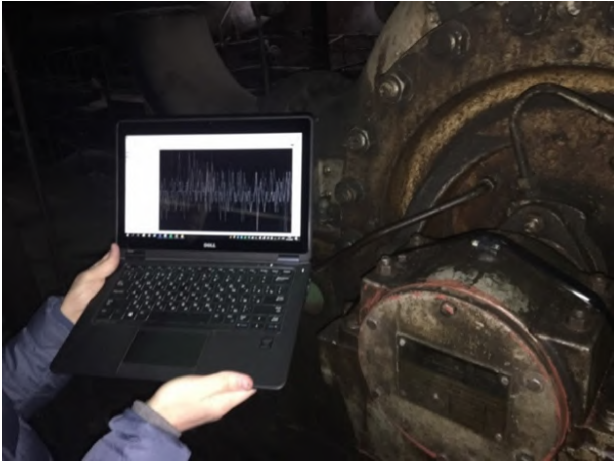
Figure 1. Vibration analysis of the auxiliary electric motor DKRAI – 4519-4V at Darnytska HPP.
