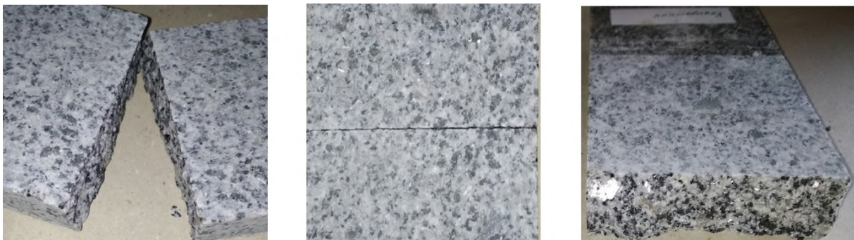
Figure 7. Example of failure in unreinforced specimens.
