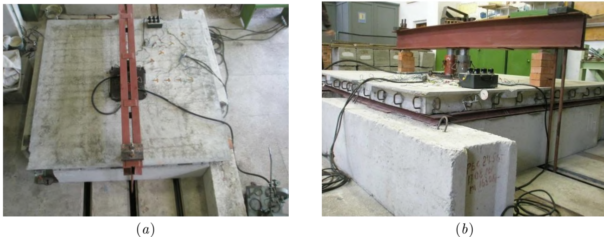
Figure 8. General view of the over-columned plate PO-1 during the test: (a) top view and (b) side view.
