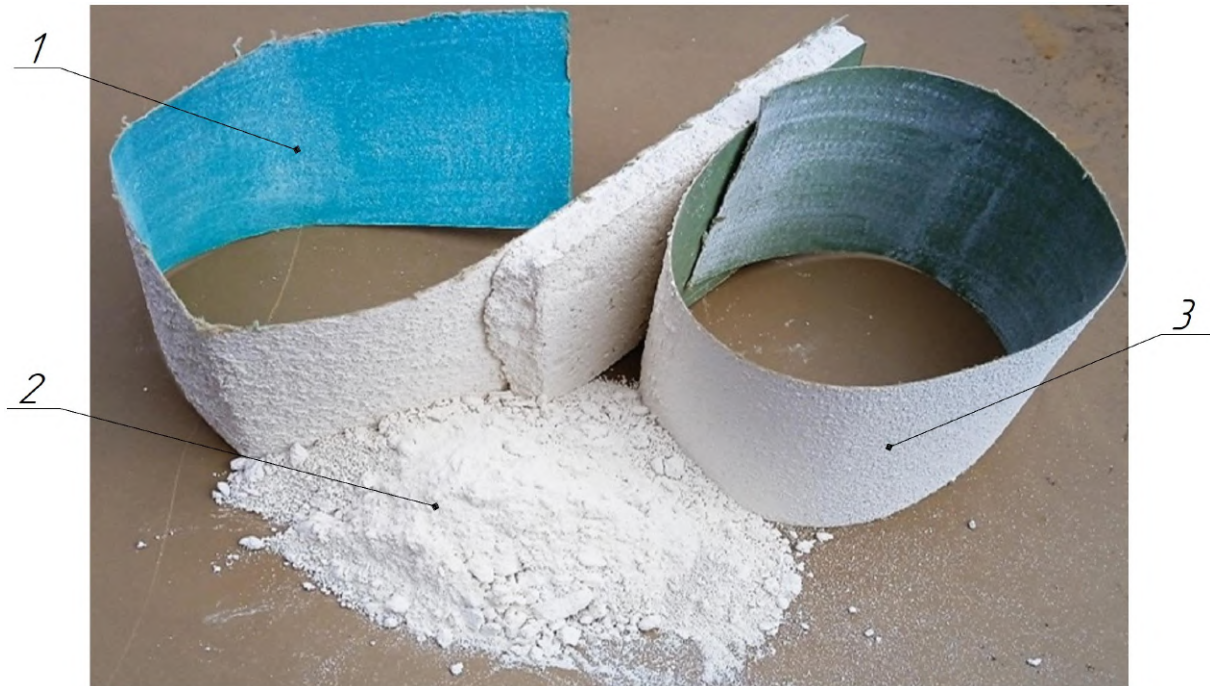
Figure 12. Drywall after high-frequency force loading: 1 – bottom plate, 2 – top plate, 3 – gypsum.
