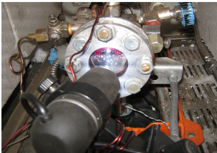
Figure 6. An example of the use of auxiliary lighting of the reactor viewing window (photo of the authors in the process of research).
