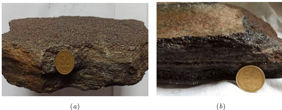
Figure 1. The most common textures of the original samples of garnet-bearing shales of the Hannivske field: (a) shale (b) shale-laminated texture.
