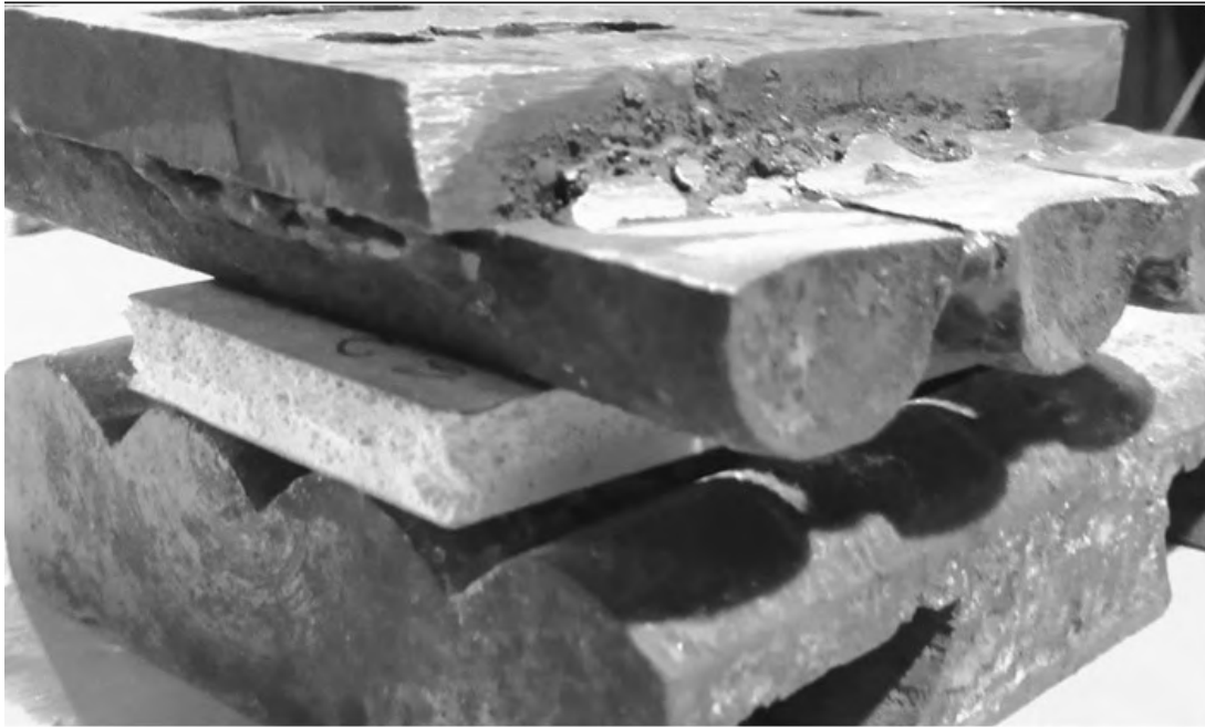
Figure 9. Oval surface profile of the lining plate.
