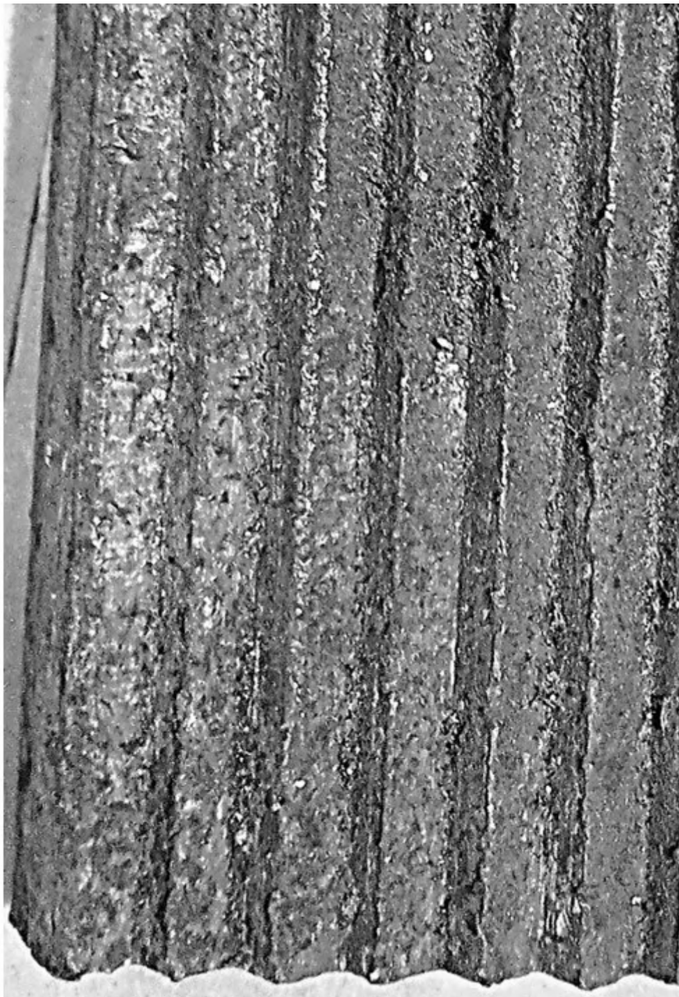
Figure 7. Prismatic surface profile of the lining plate.
