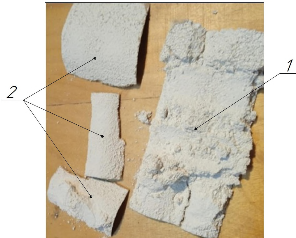
Figure 10. Crushed drywall: 1 – gypsum; 2 – cardboard.
