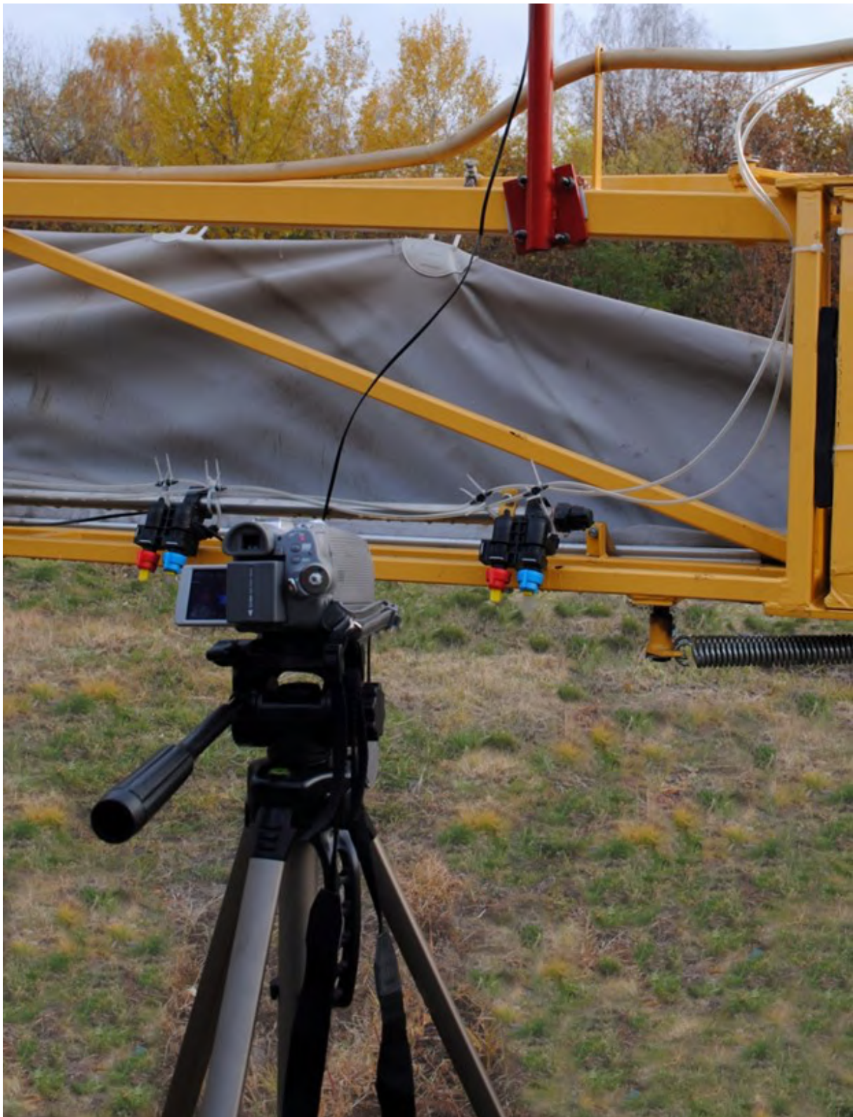
Figure 1. Filming of opening and closing of spray in flat and injector nozzles.
