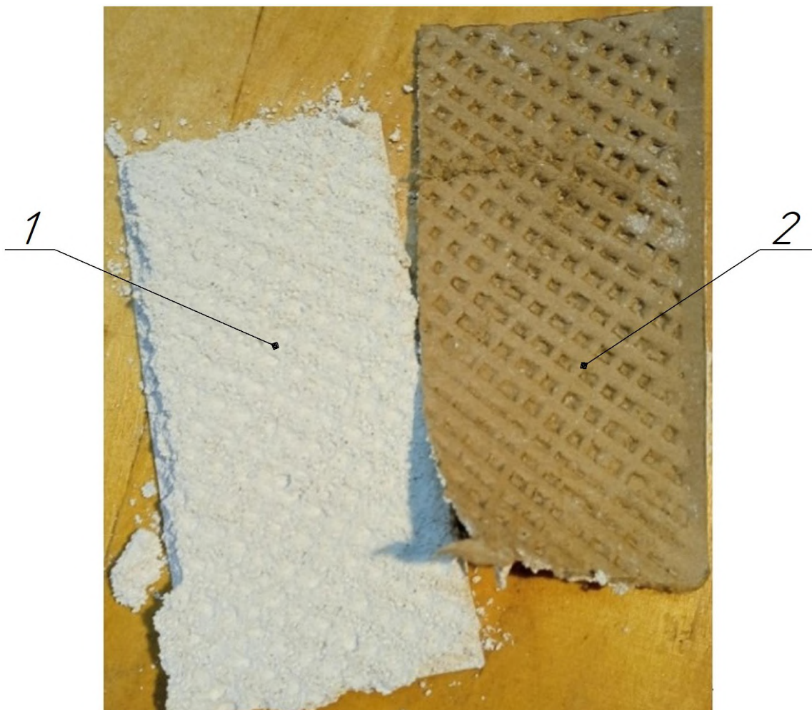
Figure 6. Crushed drywall: 1 – gypsum; 2 – cardboard.
