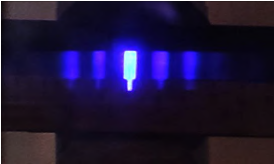
Figure 7: Real diffraction pattern.
