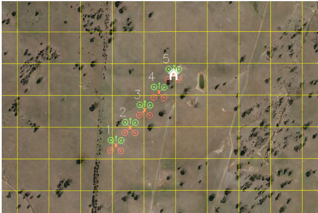
Figure 2: ArduPilot SITL Map view with multiple simulated quadcopters [16].
