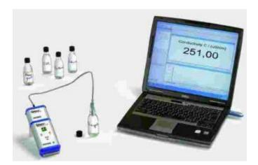
Figure 2: Investigation of the conductivity of different water samples.
