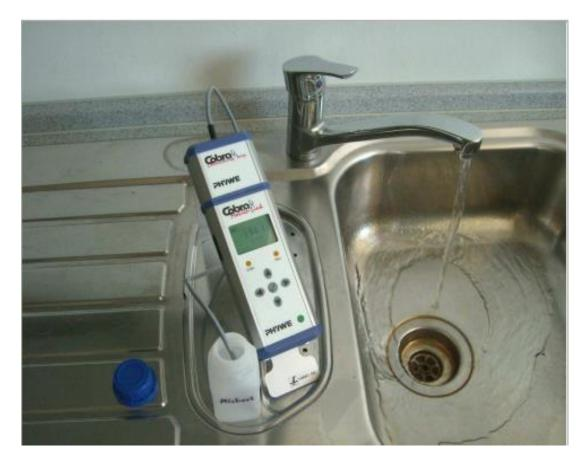
Figure 3: Measurement of conductivity values of drinking water samples at home.
