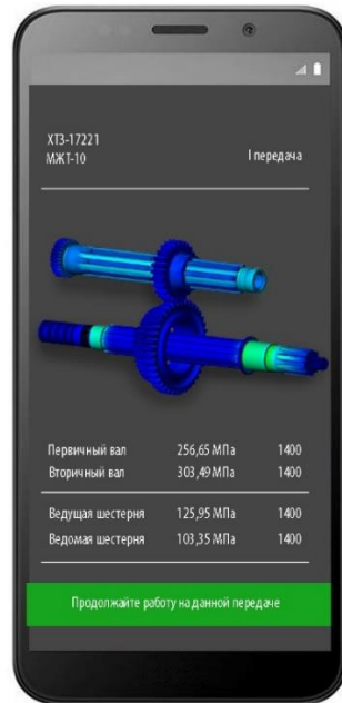
Fig. 1. General view of the application window for controlling transport-technological unit with variable mass
