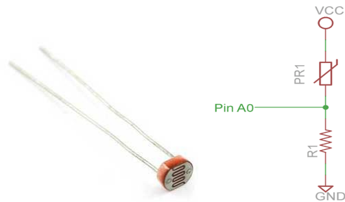
Fig. 4. Photoresistor Module Connections to Arduino.
