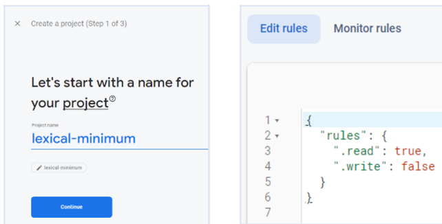
Figure 2: Register a new project in Firebase (left) and define security rules for data (right).
