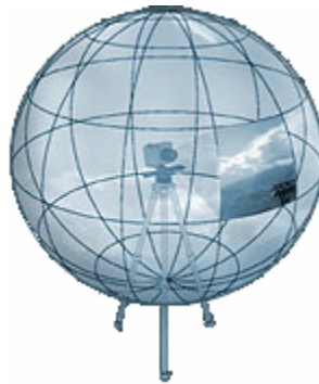
Fig. 2. The principle of composing a spherical panorama. The camera is located in the center of the field of view. A single photograph shot is shown explicitly, while for the rest, only borders are shown.
