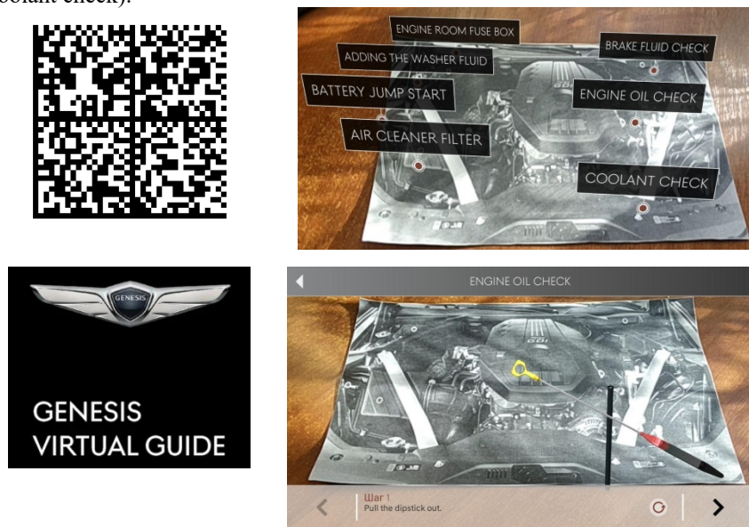
Fig. 8. Studying vehicle engine with the help of Genesis Virtual Guide app (prepared with use of [16]).
