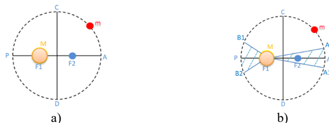
Fig. 1. Graphic representation of the first (a) and second (b) law of Kepler.
